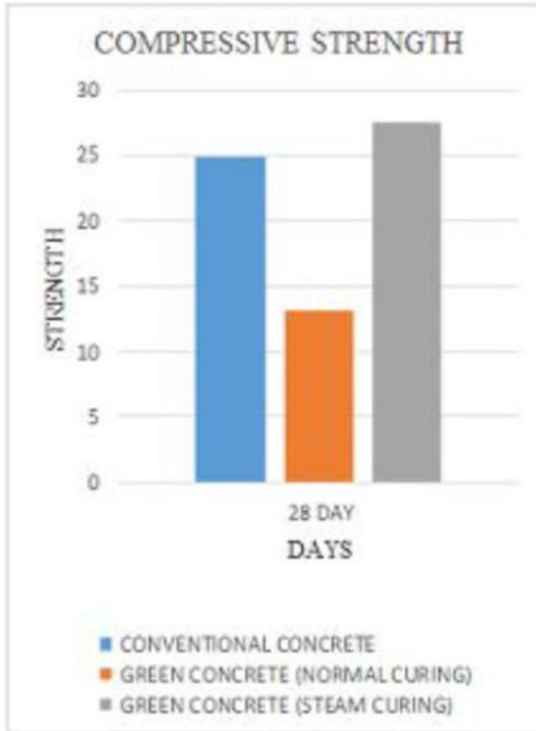
Analysis of compressive strength test result after 28 days
