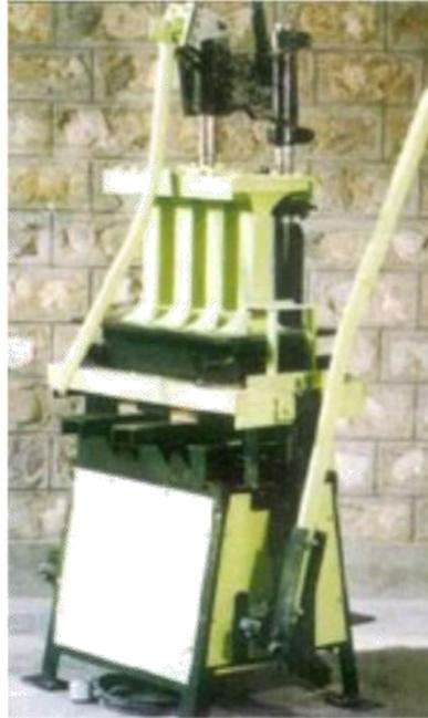
Brick pressed developed by CBRI(The engineer blog)
